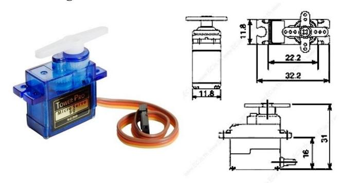
Tiny and lightweight with high output power. Servo can rotate approximately 120 degrees (60 in each direction), and works just like the standard kinds but *smaller*. You can use any servo code, hardware or library to control these servos. Good for beginners who want to make stuff move without building a motor controller with feedback & gear box, especially since it will fit in small places. It comes with a 3 horns (arms) and hardware.
