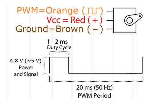
Position "0" (1.5 ms pulse) is middle, "45" ( $\sim$ 2 ms pulse) is all the way to the right, "-45" ( $\sim$ 1 ms pulse) is all the way to the left.
