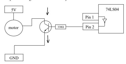
Will the motor turn when you connect the Pin 1 to 5V? Please explain with the properties of the transistor.
