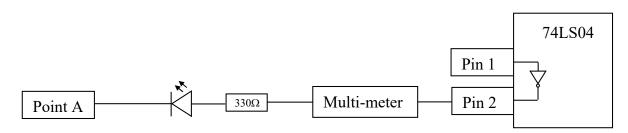
What is the current shown on the multi-meter? Is the current flowing out from Pin 2 or flowing into the Pin 2?
