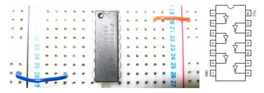
3. Connect Pin 1 to GND, measure the voltage at Pin 2. What is the voltage at Pin 2?
