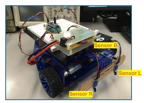
You need to include the bumper sensor (**Sensor B to A4**) into your circuit and to write in the coding text template given at Lab#06
