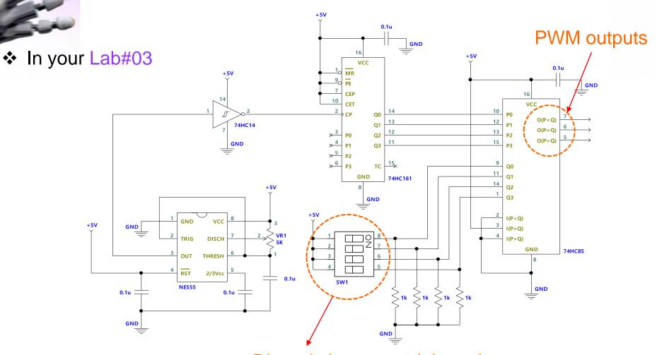
Dip switch to control the value of 74HC85 input
