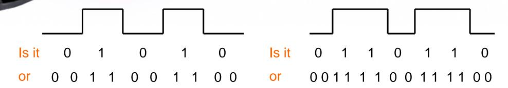
❖ A synchronization signal called a "clock" is needed
