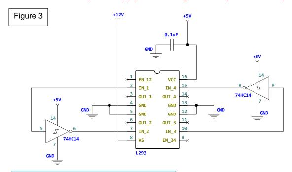
**74HC14** is the Schmitt-Trigger Inverter you used in Lab3. As shown in the illustration, there are six inverters inside the package and they are independent to each other. You may choose whichever is available and convenient according to your breadboard layout.
