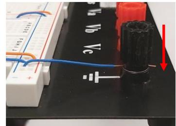
3. Screw tight the housing. Make sure that the wire's insulator is not grabbed.
