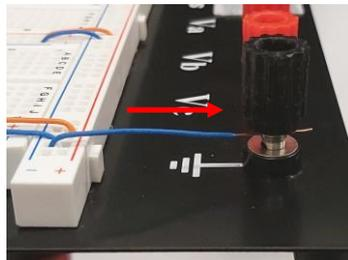
2. Insert wire into the hole. Note the openings of the wire is ~15mm.
