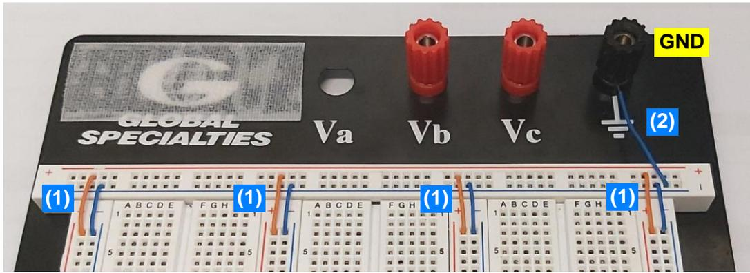
Step 2: Connect a wire from the GND row of the bus strip to the black binding post.
