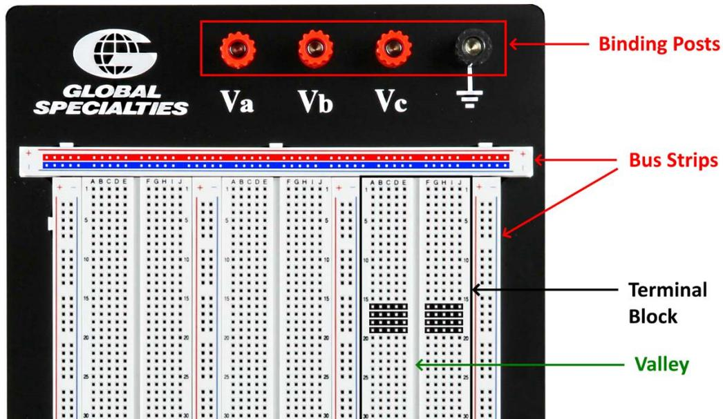
The **binding posts** are usually used to connect to different power sources.
