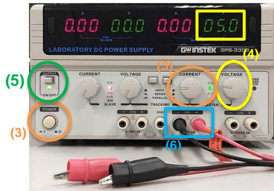
Step 3: Switch on the power supply. Select one variable channel and slowly turn its “CURRENT” knob clockwise until the marking line on the knob is horizontal and the CV light (green) is on. **CV stands for Constant Voltage. This is an important step to protect your circuit by limiting the output current from the power supply.**
