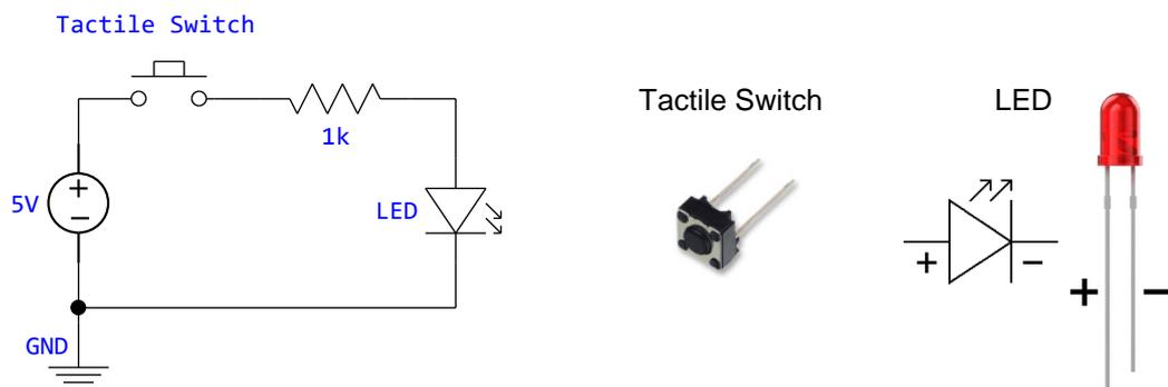
Step 2: While observing the LED, press and release the tactile switch.
