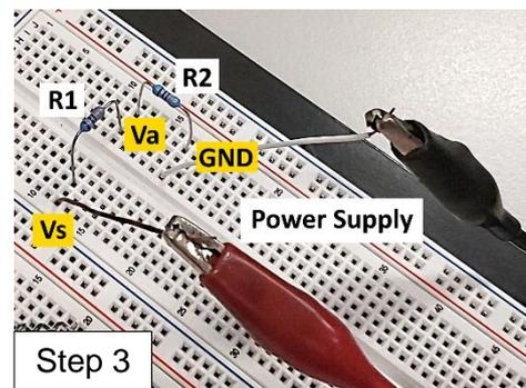
Step 3: Switch off the power supply and turn all the knobs fully anticlockwise as in **Experiment 3**. Connect a variable output channel (Master or Slave) to the resistors accordingly.
