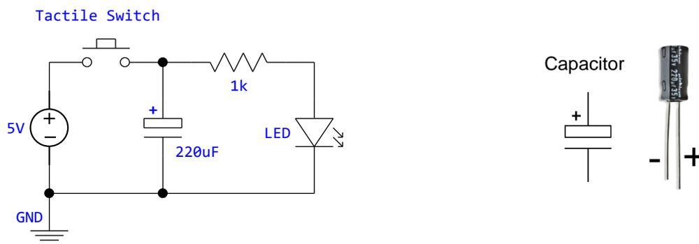
Step 4: While observing the LED, press and release the tactile switch.
