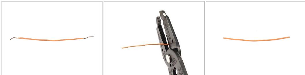
Step 2: There are several stripping holes on the wire stripper. One of the two holes on top shall be good for our provided wires. (a) "Seat" the wire into one side of the proper hole. The cut end shall be **~7mm** from the hole. (b) Slowly press the handles together. (c) Pull the wire stripper towards the cut end of the wire to remove the insulation. (d) Use the scale on stripper to verify the length of the openings.
