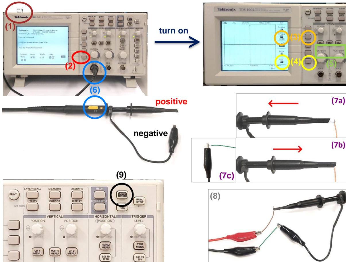
Step 6: Connect the DSO Probe head to the oscilloscope and set the probe to 1X.
