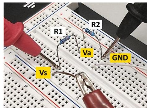
Also, the probe lead should touch at the pin bottom of the resistor (or other components) for a stable contact.
