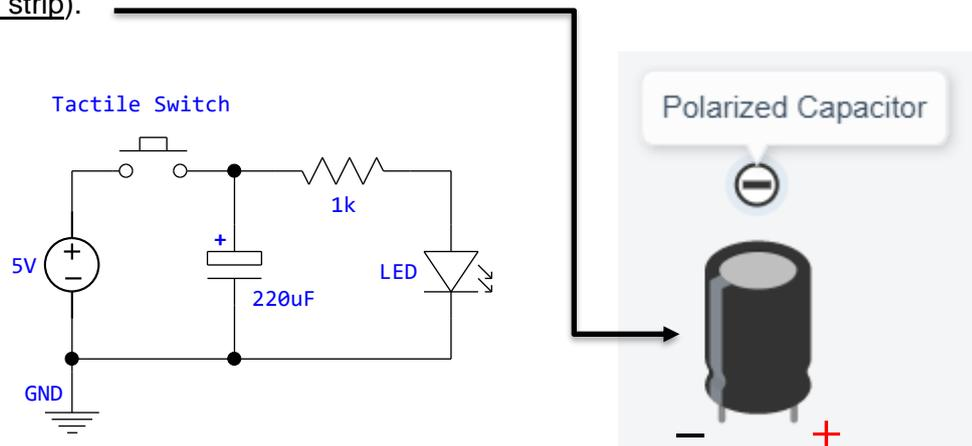
Step 5: Set power supply to be 5V, capacitance to be 220uF in Tinkercad.
