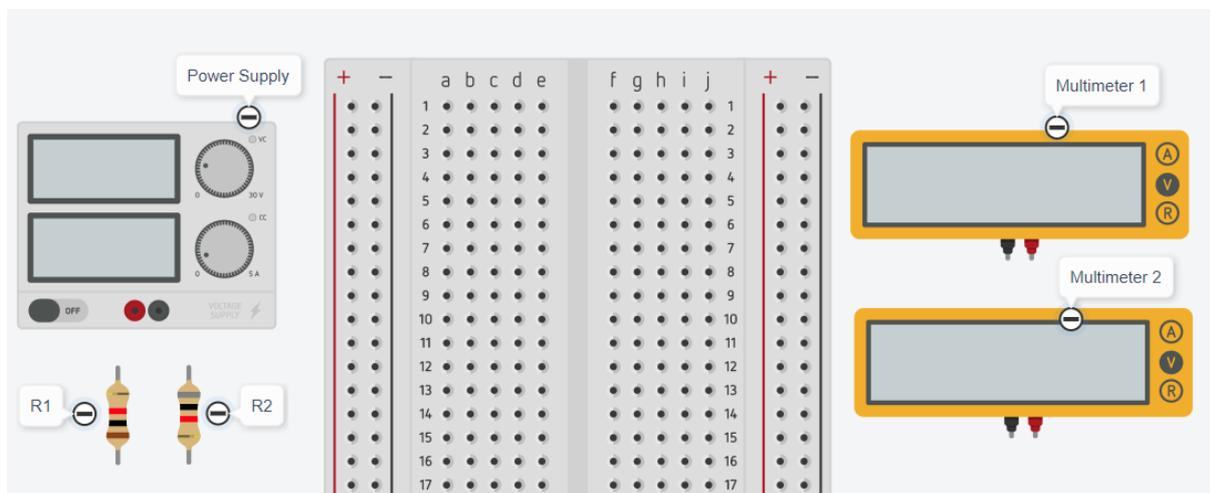
Step 1: Create a new circuit in **Tinkercad** and change the circuit name. Find components as needed.
