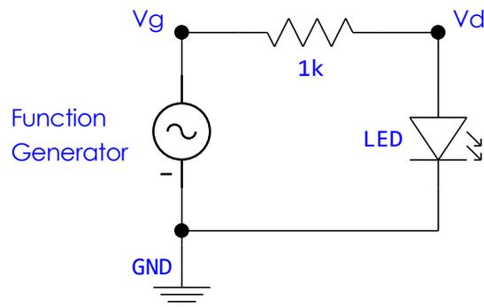
Step 2: In this experiment, you need two Oscilloscopes. Use Oscilloscope 1 to measure Vg and Oscilloscope 2 to measure Vd.
