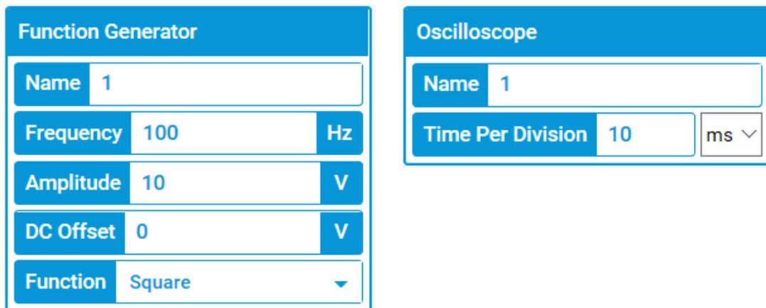
**Note:** In Tinkercad, the value of “Amplitude” = Vpp (peak to peak value).
